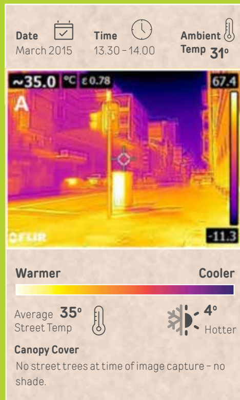
Figure 22. Terrestrial thermal imaging of three city streets
