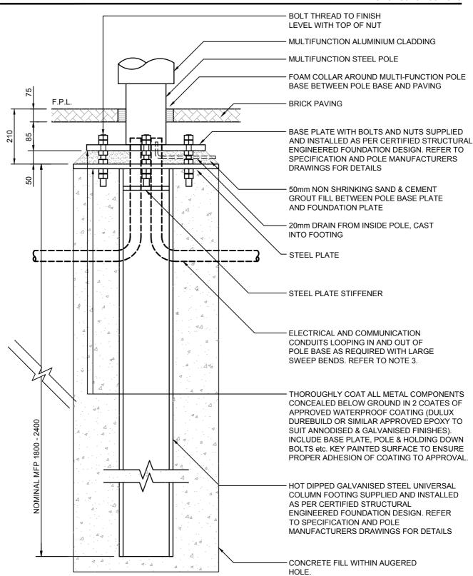
Note: Pole foundations to be structurally designed and certified by practicing structural engineer in accordance with site conditions, Australian standard and manufacturers recommendations. Submit shop drawings and structural engineered certification for review prior to manufacture and installation.
