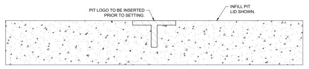
PIT LOGO IS TO BE INSTALLED INTO THE WET IN-SITU CONCRETE IN THE INFILL PIT LID.
