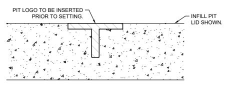
PIT LOGO IS TO BE INSTALLED INTO THE WET IN-SITU CONCRETE IN THE INFILL PIT LID.
