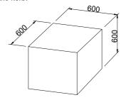
In rare cases, where circumstance does not allow a depth of 400mm (e.g. because of drains or cables), depth can be reduced to 400mm, providing the widths are increased to 800mm)
