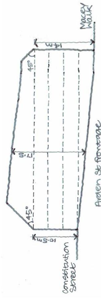
Figure 3: - Building envelope for Lot 9
